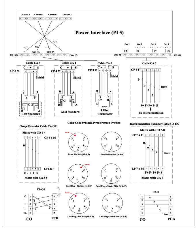
6.5 Terminators are special connectors with circuitry to connect to the inputs of any unused channels. These provide the proper connections to conditioner electronics so that improper terminations are eliminated. Failure to use these connectors can result in failure of the circuitry of a conditioner.
