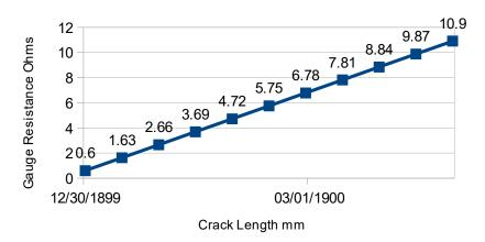
Let us assume that a 100 DCB gauge is to have it's active crack length space reduce from 105 to 60 mm. The active length of 60 mm will give a smaller nonlinearity at 100% than the standard 100 DCB gauge which only has an excess of 5 mm. (Assumption #1)
